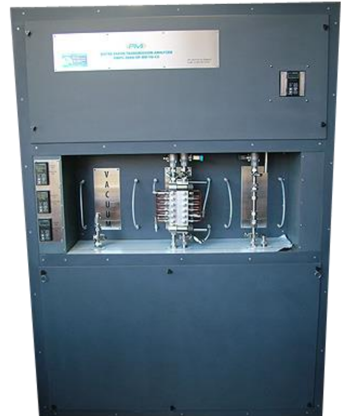
PMI Water vapor transmission analyzer for membrane distillation
